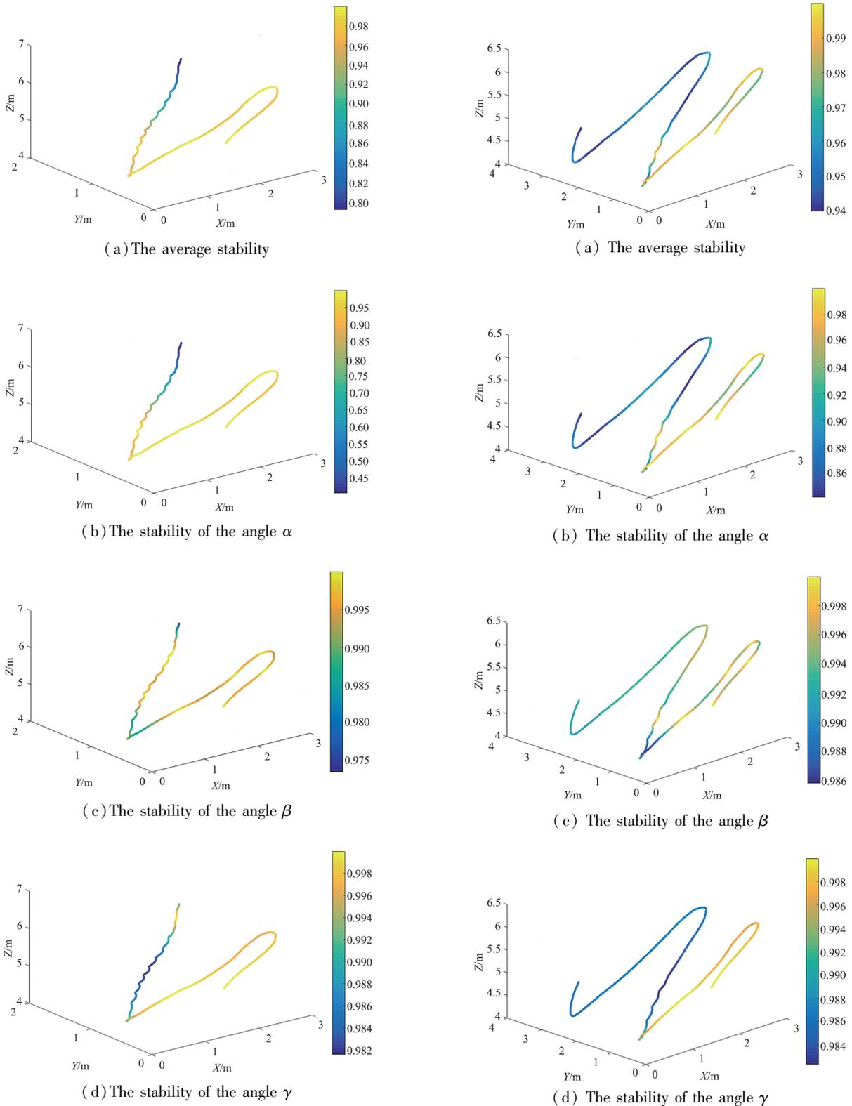
**Fig. 4** Stability of the suspended object with the motion trajectory before trajectory planning
