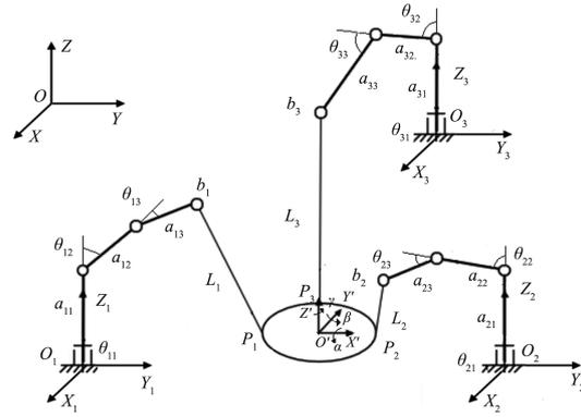
Fig. 1 The structure of the towing system
