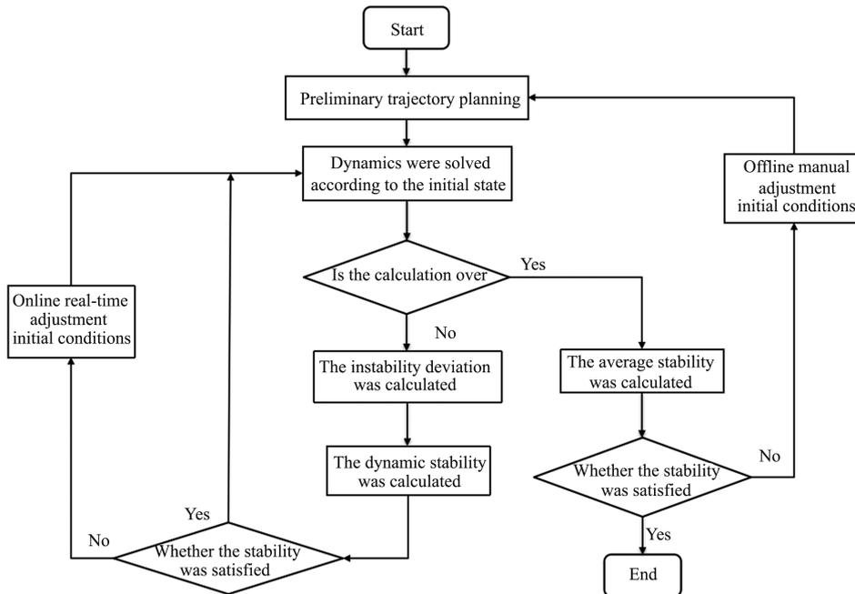
Fig. 2 Flowchart of the trajectory planning
