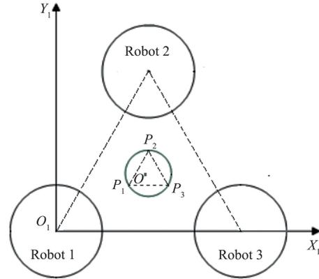
Fig. 3 Projection of the towing system on the XOY plane
