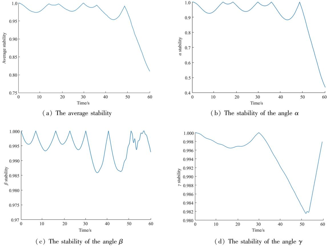
**Fig. 6** Stability of the suspended object over time before trajectory planning
