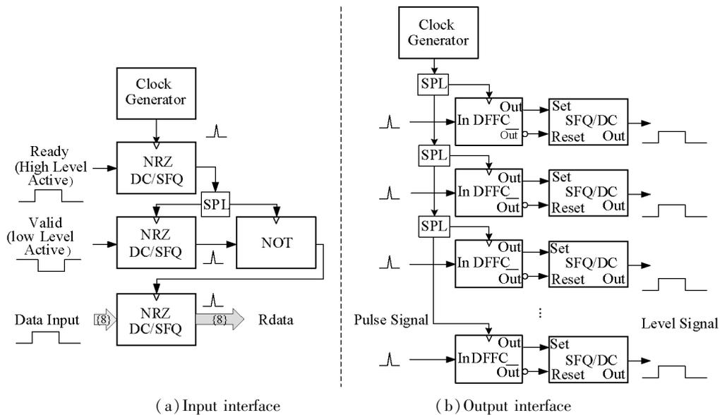
Fig. 9 Logic diagram of superconducting RSFQ circuit
