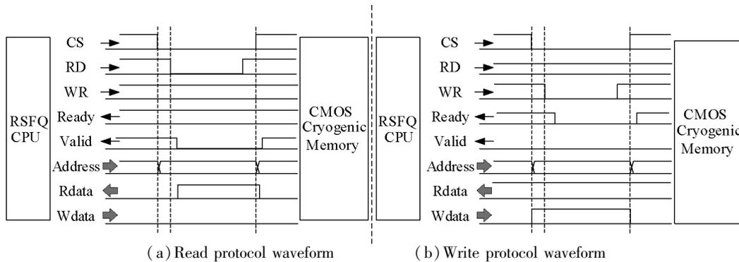
Fig. 8 Working waveforms of the asynchronous communication protocol
