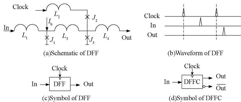
Fig. 5 Schematic diagram of DFF cell
