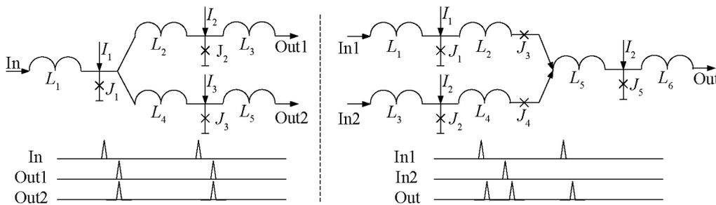
Fig. 3 Schematic diagram of SPL and CB
