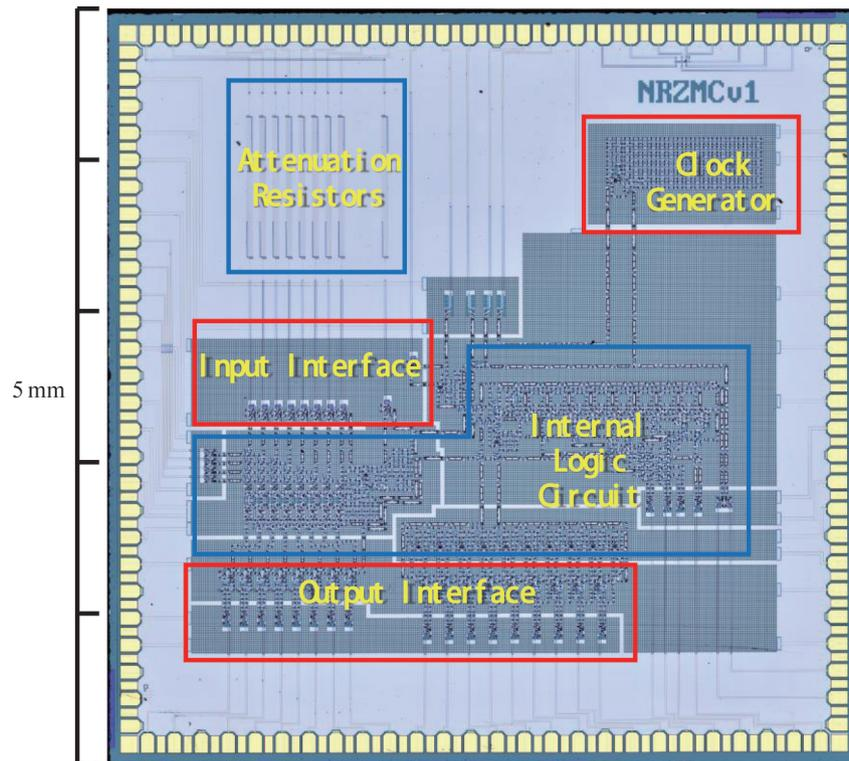
**Fig. 12** Superconducting RSFQ CPU test chip physical layout
