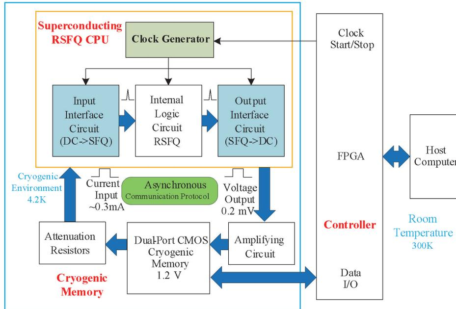
Fig. 6 Architecture of superconducting RSFQ circuit control system
