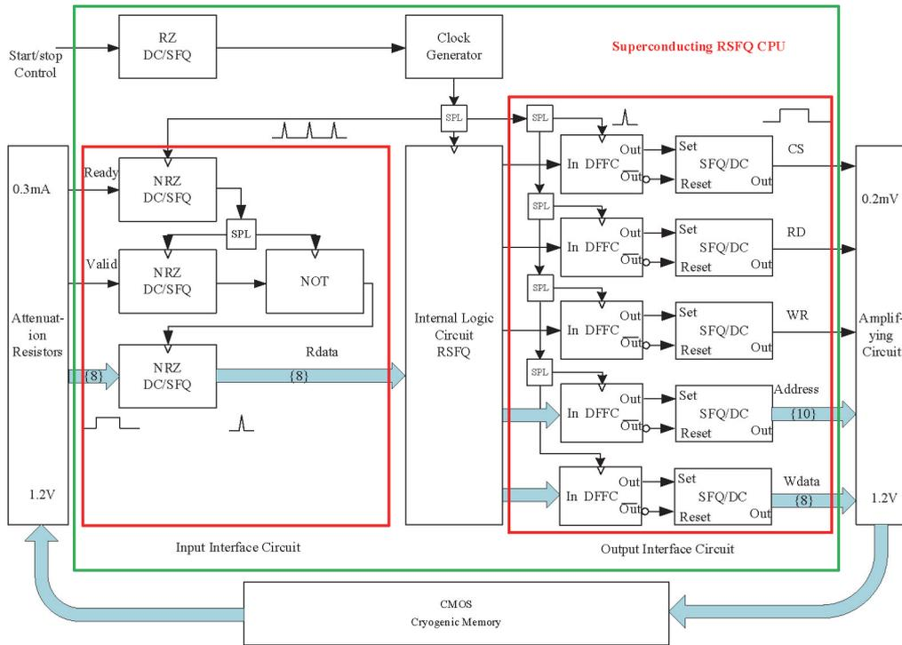
Fig. 10 Logic diagram of asynchronous communication circuit
