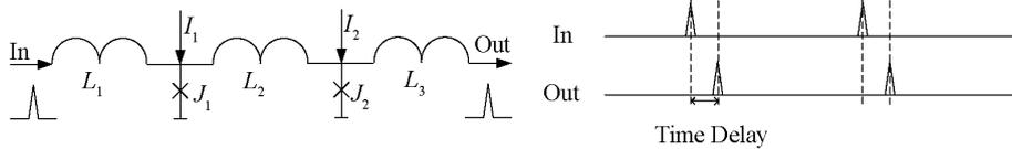
Fig. 2 Schematic diagram of a Josephson transmission line (JTL)
