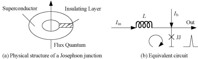
Fig. 1 Schematic diagram of JJ
