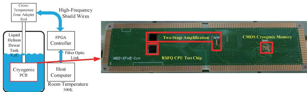
Fig. 11 Overview of the proposed superconducting RSFQ circuit control system
