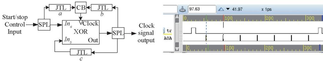
(a) Logic diagram of RSFQ clock generator (b) Waveform of RSFQ clock generator
