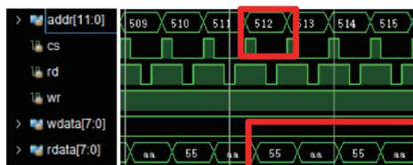
(c) Reading data after testing chip operation
