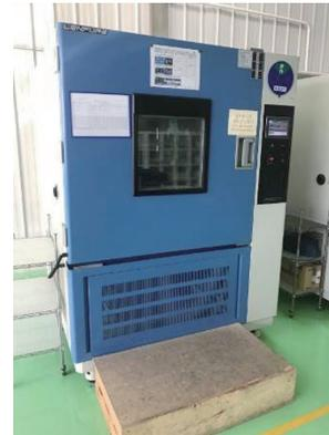
**Fig. 21** High and low temperature test chamber
