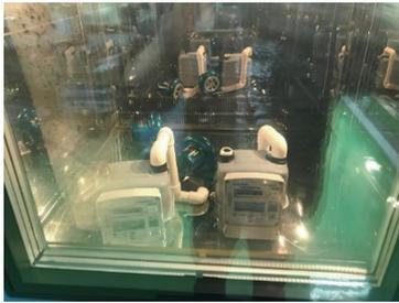
(b) High and low temperature endurance testing device
