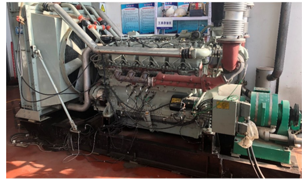
Fig. 11 Diesel engine fault simulation test bench
