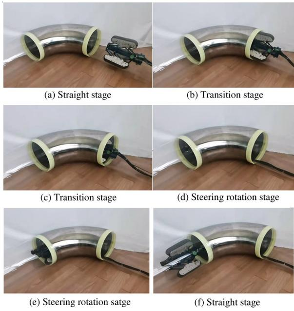
Fig. 13 Robot steering motion experiment process
