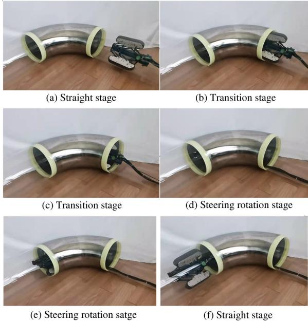
**Fig. 13** Robot steering motion experiment process
