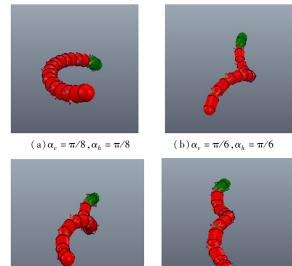
(c)  $\alpha_v = \pi/4$ ,  $\alpha_h = \pi/4$  (d)  $\alpha_v = \pi/2$ ,  $\alpha_h = \pi/2$ **Fig. 7**  $\alpha_v$  and  $\alpha_h$  under different radius of a spiral
